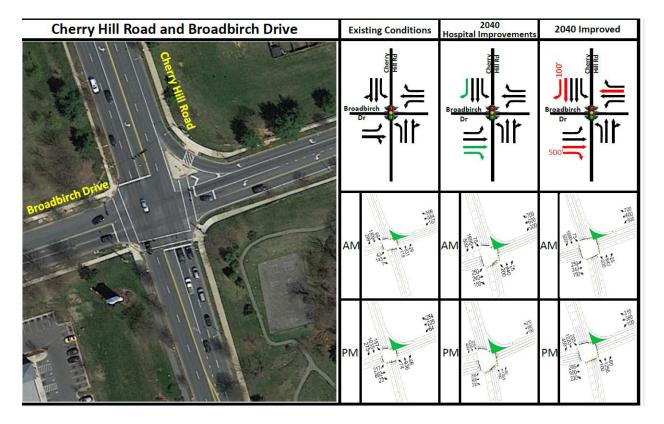
Using the 2040 Improved diagram, a dedicated right-turn lane and another thru-lane from Broadbirch needs to be added, a right-turn lane from eastbound Cherry Hill needed to be added and a second thrulane from Calverton Blvd needs to be added. This configuration would require either adding a lane or eliminating the parking on the east side of the Calverton Blvd between Cherry Hill Rd and Gracefield Rd.
